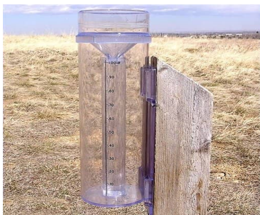
Figure 1. (a) An ordinary rain gauge with an outer rim 11.28 cm in diameter and a laboratory cylinder graduated in cubic centimeters and (b) an automatic model is used to measure precipitation.
